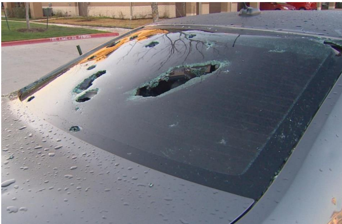
Figure 3-45: Hail damage after a March 2019 storm in the DFW area. 210
