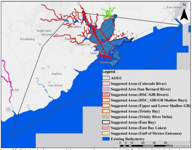
Figure 33. Existing bathymetry and the suggested area to acquire bathymetric data based on data availability of year of last acquisition for AOI 11. Please also refer to AOI 4, 7, and 13 for more information on some of the suggested areas shown here and not listed under AOI 11. Different hatched colors are not clearly distinguishable tin the figure to the number of active layers. All the GIS files can be found <u>here</u>.
