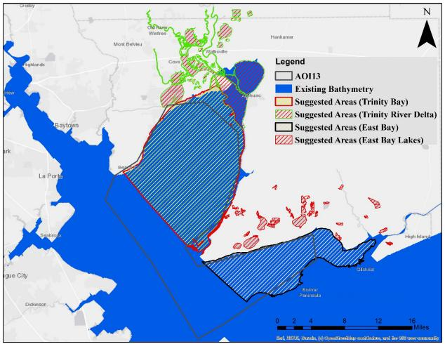
Figure 36. Existing bathymetry and the suggested area to acquire bathymetric data based on data availability of year of last acquisition for AOI 13. Please also refer to AOI 4, 7, and 11 for more information on some of the suggested areas shown here and not listed under AOI 13. Different hatched colors are not clearly distinguishable tin the figure to the number of active layers. All the GIS files can be found <u>here</u>.
