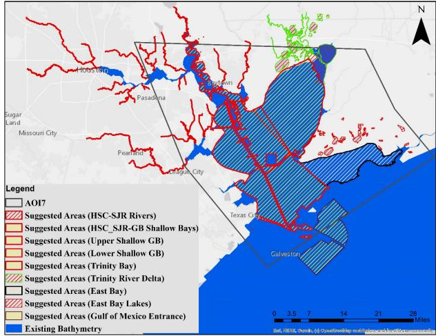
Figure 24. Existing bathymetry and the suggested area to acquire bathymetric data based on data availability of year of last acquisition for AOI 7. Please also refer to AOI 4, 11, and 13 for more information on some of the suggested areas shown here and not listed under AOI 7. Different hatched colors are not clearly distinguishable tin the figure to the number of active layers. All the GIS files can be found <u>here</u>.
