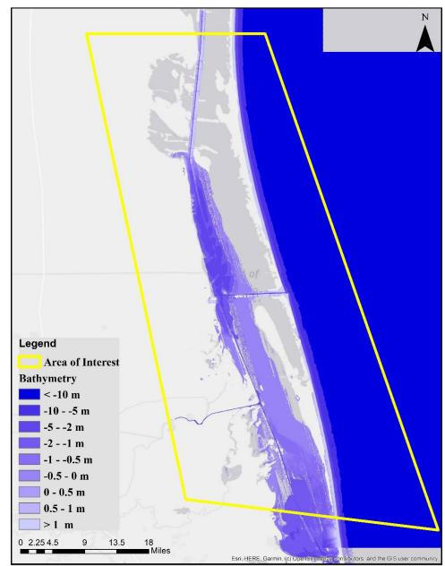
Figure 19. Bathymetry of AOI 6 using the BlueTopo and the 2 extra TWDB databases.
