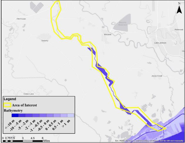
Figure 3. Bathymetry of AOI1 using the BlueTopo database.
