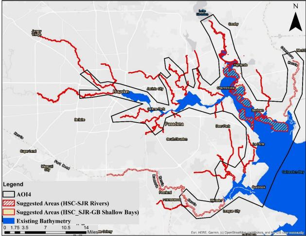
Figure 14. Existing bathymetry and the suggested area to acquire bathymetric data based on data availability of year of last acquisition for AOI 4.
