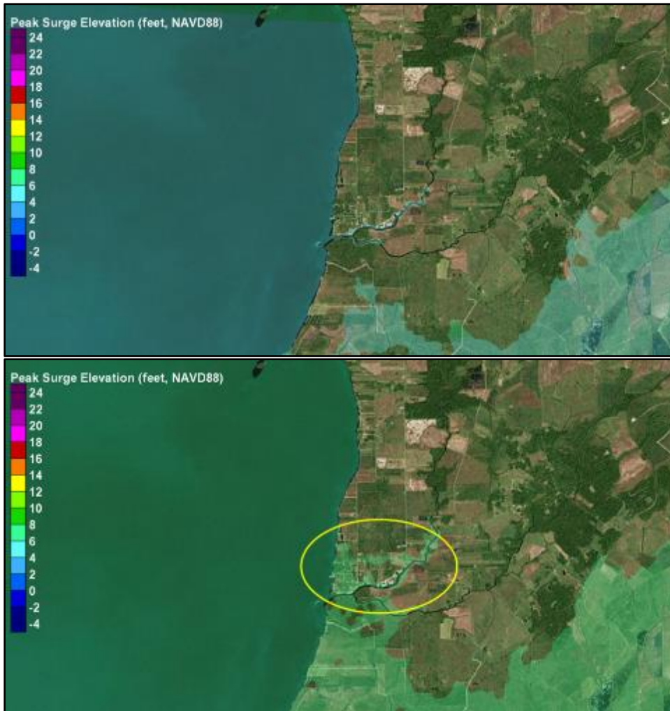
Figure 15. Inundation Maps for the Town of Oak Island, for Hurricane Ike and Future Sea Level, for the Ike Dike Coastal Spine Concept having a Western Section (top panel) and an Alignment Similar to the Likely USACE TSP that does not have a Western Section (bottom panel).
