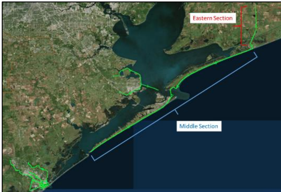
Figure 17. Alignment of the Coastal Spine Similar to that Recommended by the USACE in the Coastal Texas Study as Part of Alternative A, the Likely TSP, for the Houston Galveston region.
