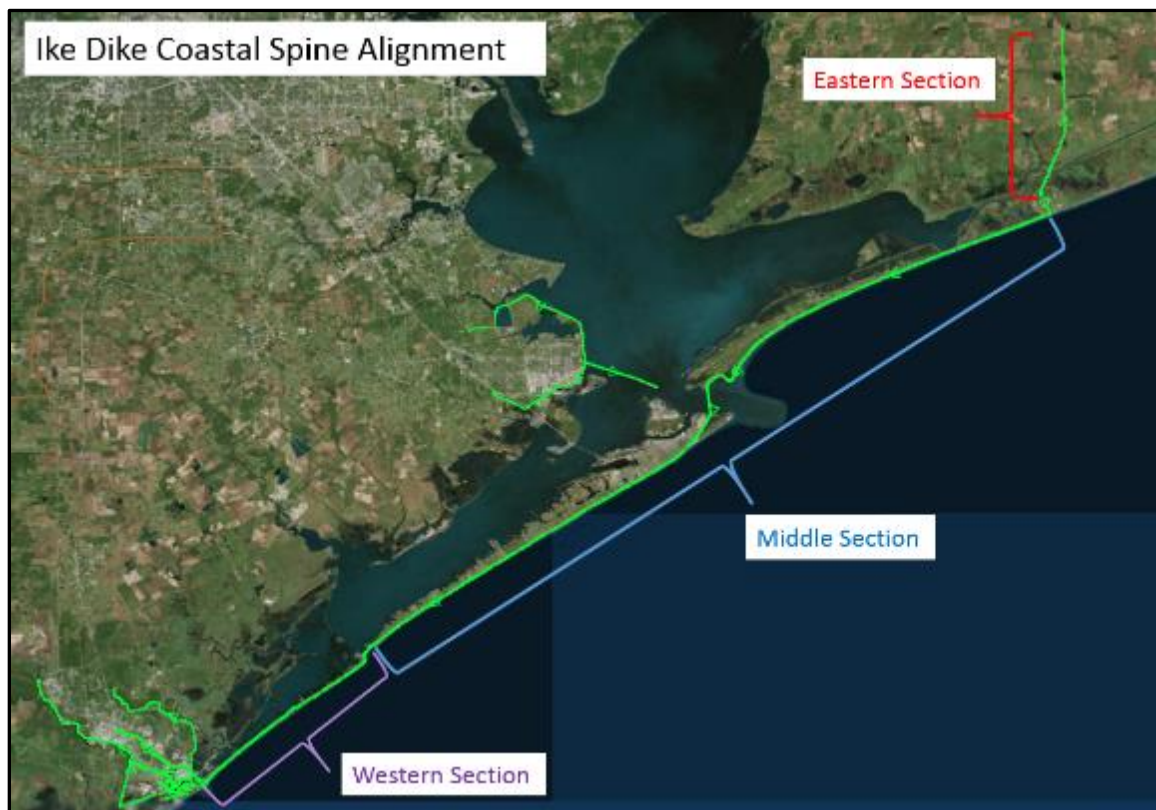
Figure 1. Current Alignment of the Ike Dike Coastal Spine Concept Proposed by TAMUG and its Research Collaborators.
